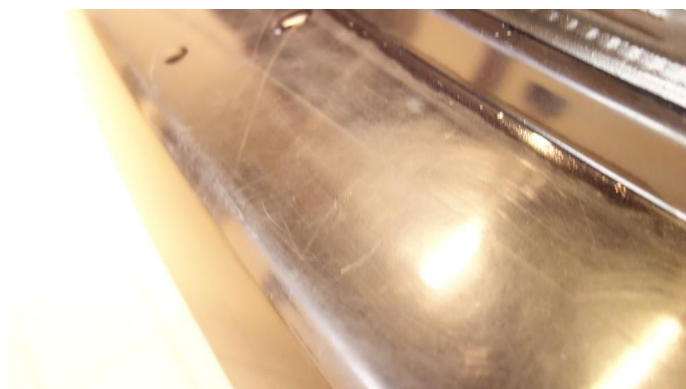
1.1 Riper innlasting baggagerom poleres
