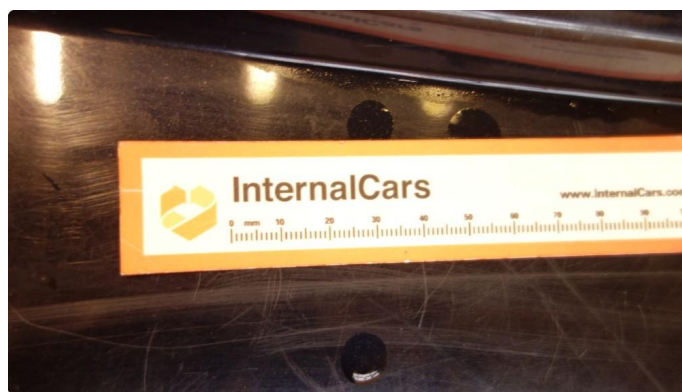
1.1 Riper innlasting baggagerom poleres
