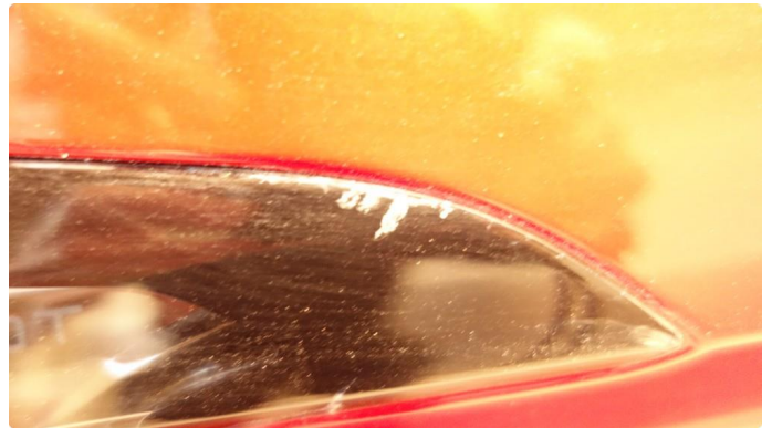
2.1 Krakelering i plast
