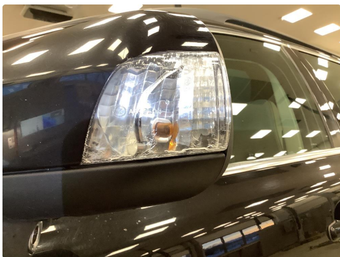
2.1 Krakelering i plast
