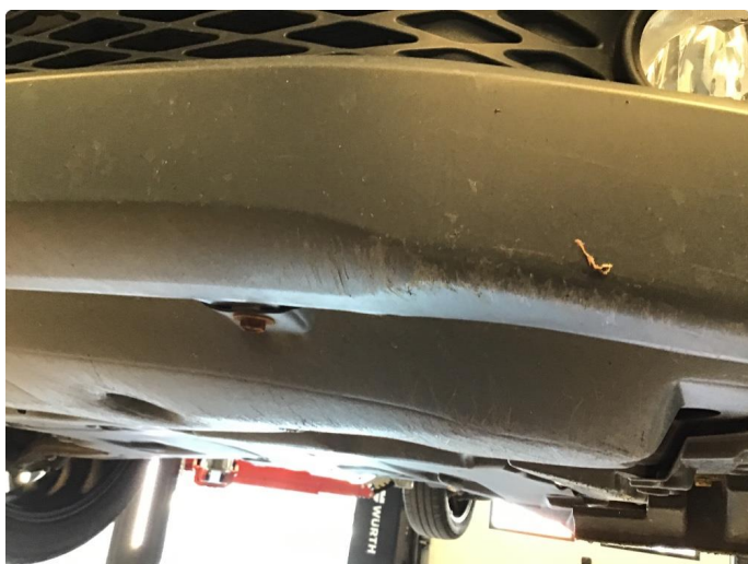
1.7 Skrubbeskader under frontfanger
