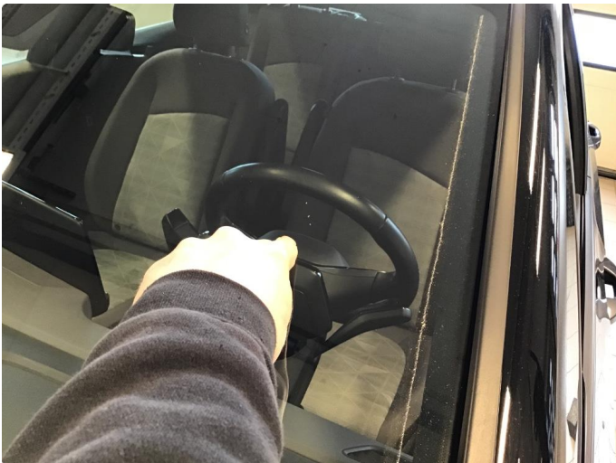
1.2 Steinsprut i synsfelt
