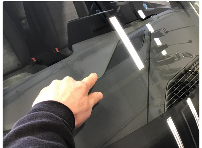
1.2 Steinsprut i synsfelt
