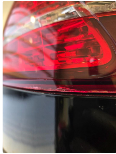
2.1 Krakelering i plast
