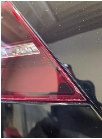
2.1 Krakelering i plast
