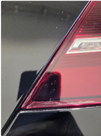
2.1 Krakelering i plast
