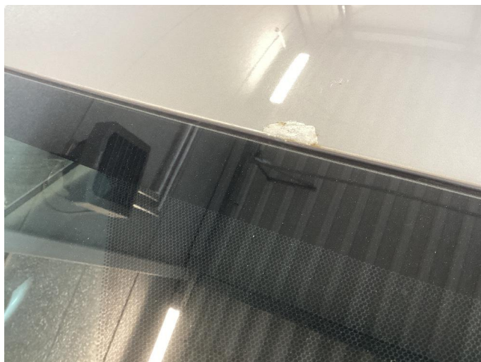
1.4 Noe rust p tak over frontvindu
