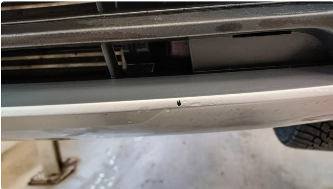
1.1 Liten steinsprut i fanger foran. Lakkeres forenklet
