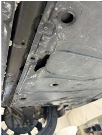
1.1 Liten sprekk i plate under bil
