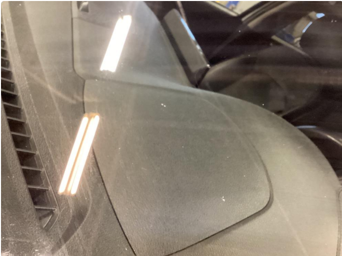
1.3 Steinsprut utenfor synsfelt
