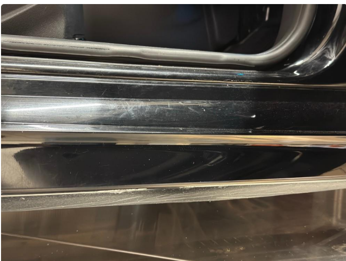
1.5 Slitt lakk innsteg
