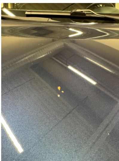
1.2 Diverse lakkskavanker / rust
