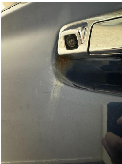
1.2 Diverse lakkskavanker / rust
