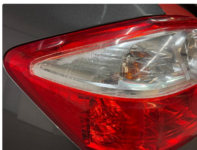
2.1 Krakylerte lamper / fukt
