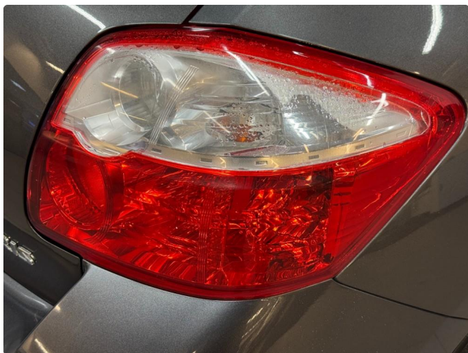
2.1 Krakylerte lamper / fukt
