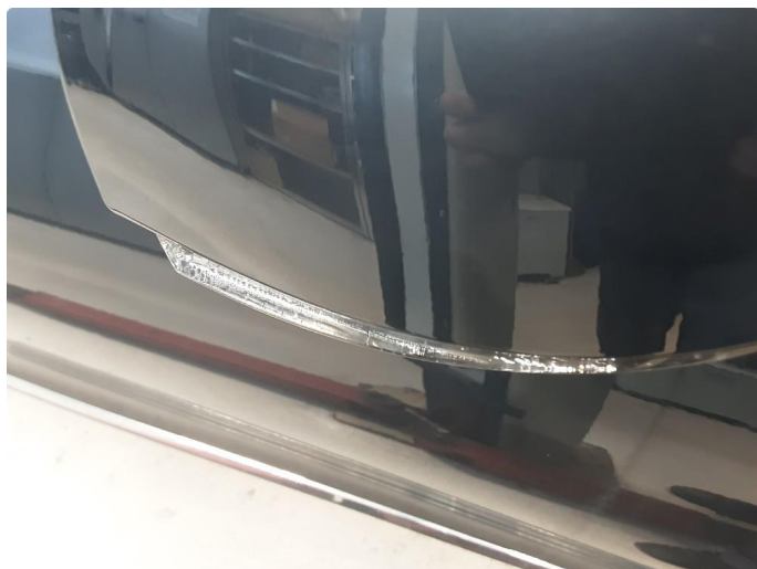
2.1 Krakelering i plast
