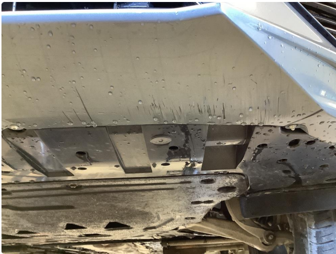
1.3 Noe skrubbskader underkant
