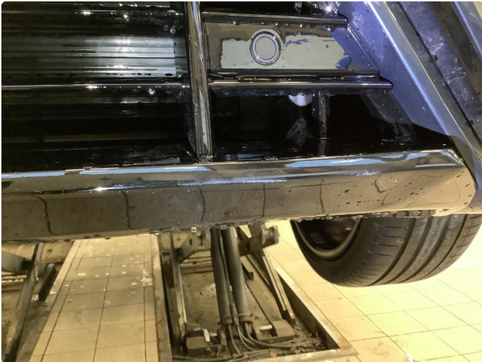
1.1 Noe skrubbskader underkant
