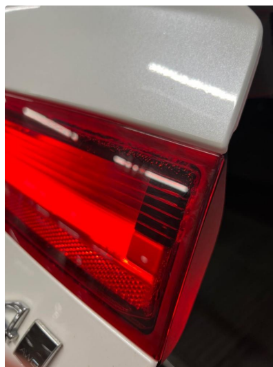
2.1 Krakelering i plast
