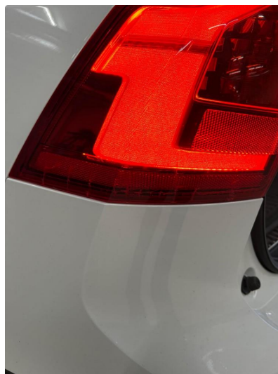
2.1 Krakelering i plast
