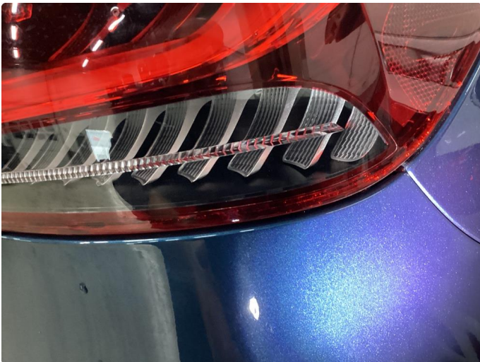
2.1 Krakelering i plast
