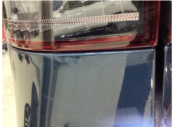
2.1 Krakelering i plast
