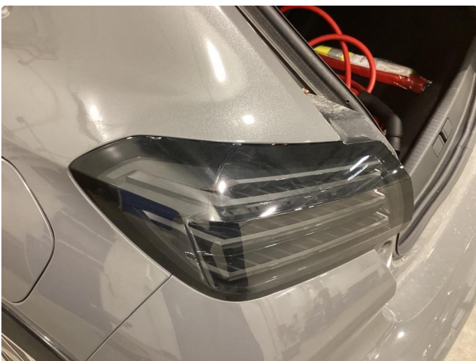
2.1 Krakelering i plast
