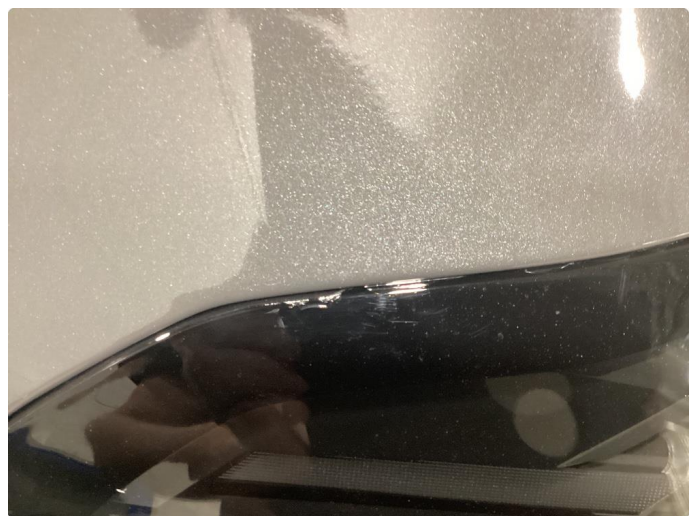
2.1 Krakelering i plast
