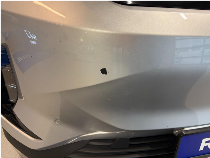
1.1 Steinsprut i frontfanger
