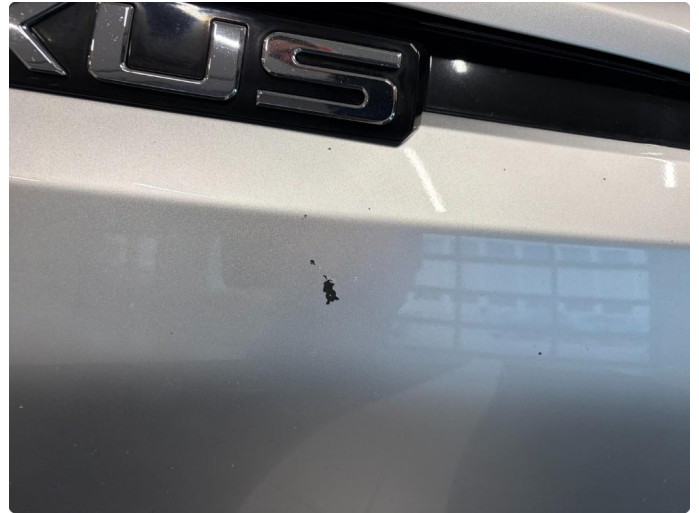
1.1 Steinsprut i frontfanger
