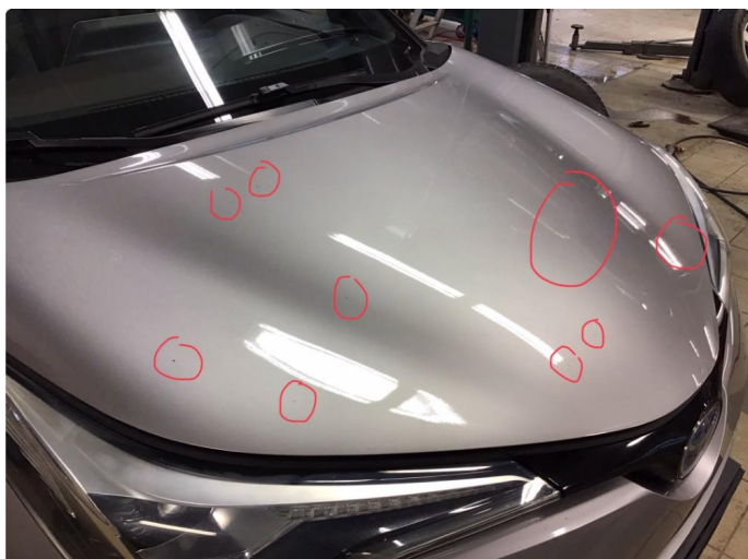
1.1 Noe stensprut i front.
