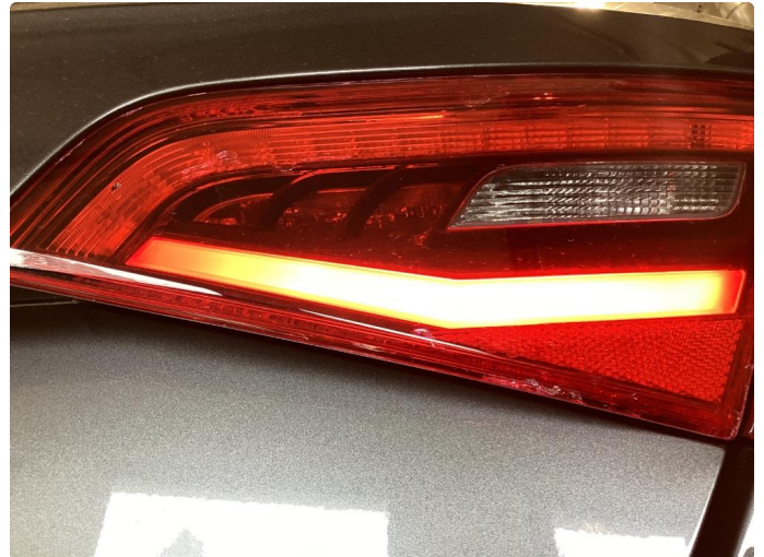
2.1 Krakelering i plast
