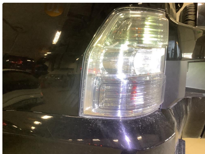
2.1 Krakelering i plast
