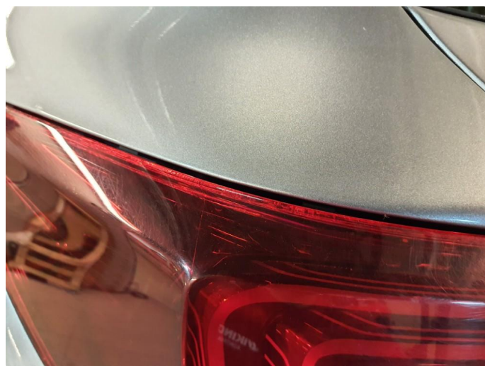
2.2 Krakelering i plast
