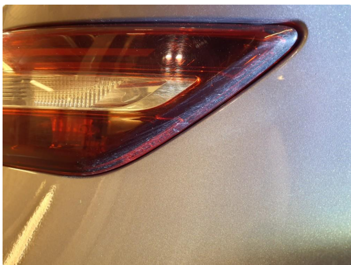
2.2 Krakelering i plast
