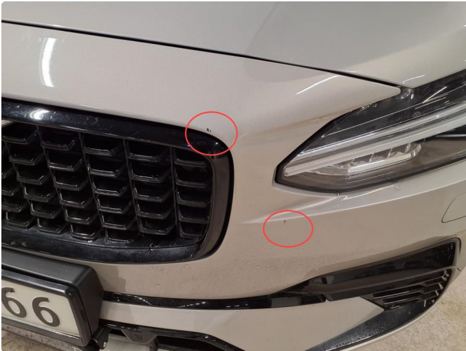
1.1 Noe steinsprut frontfanger
