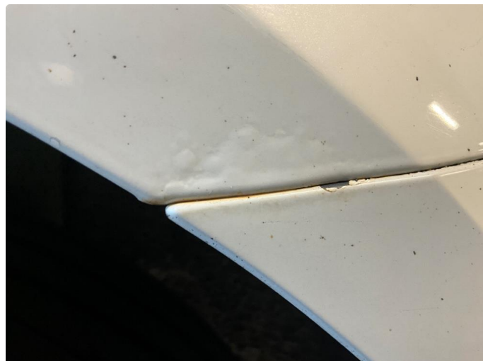
1.1 Rust i fals.
