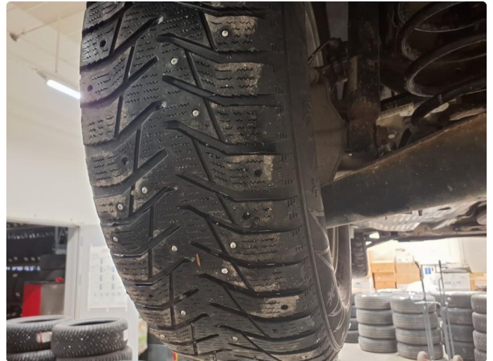
1.3 Piggdekk mangler pigger. 215/65R16
