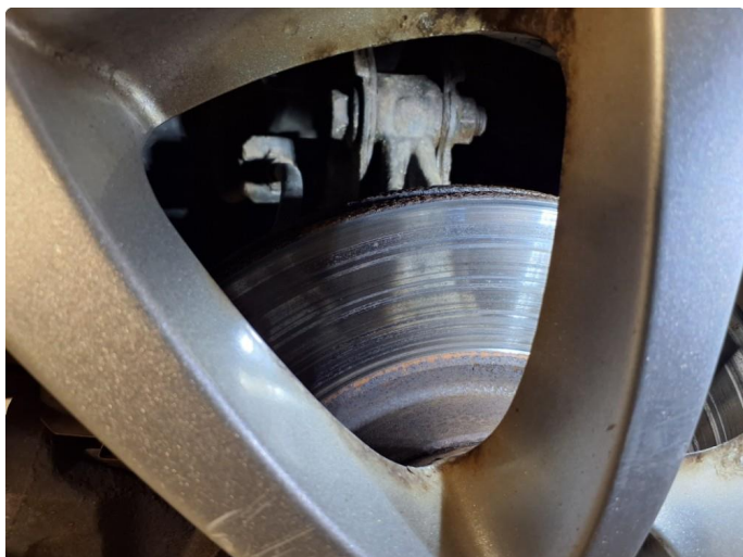
5.1 Mer enn 25% rust
