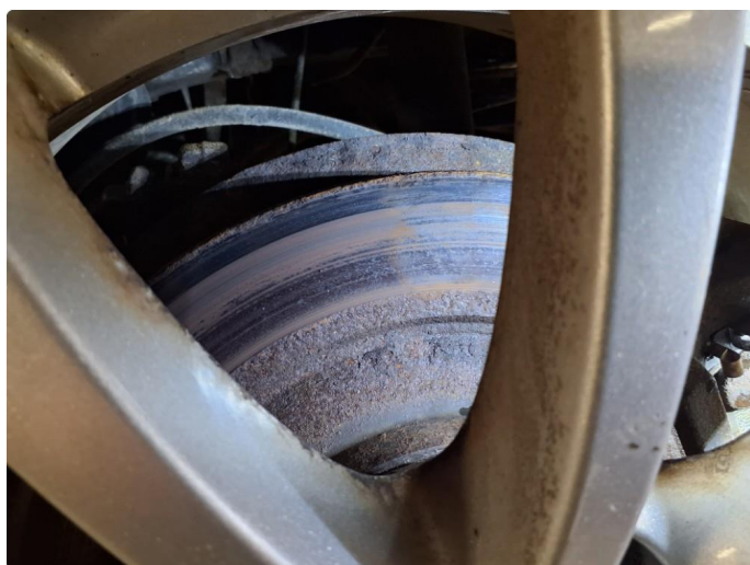
5.1 Mer enn 25% rust
