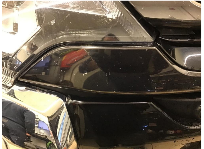
1.1 Noe lakklass grill pga steinprut.
