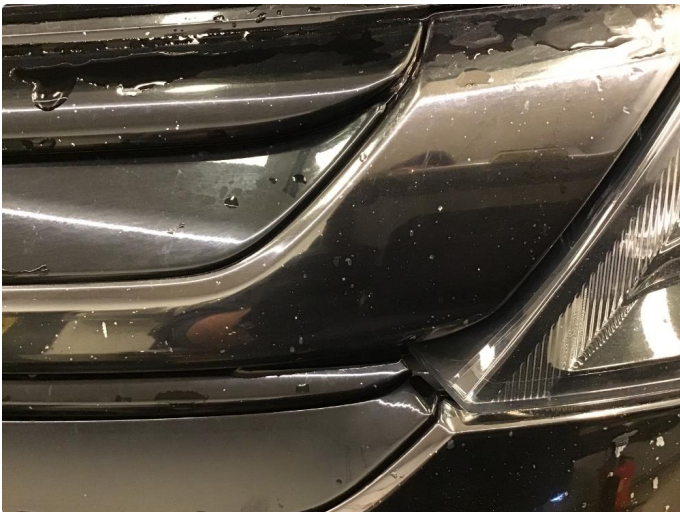
1.1 Noe lakklass grill pga steinprut.
