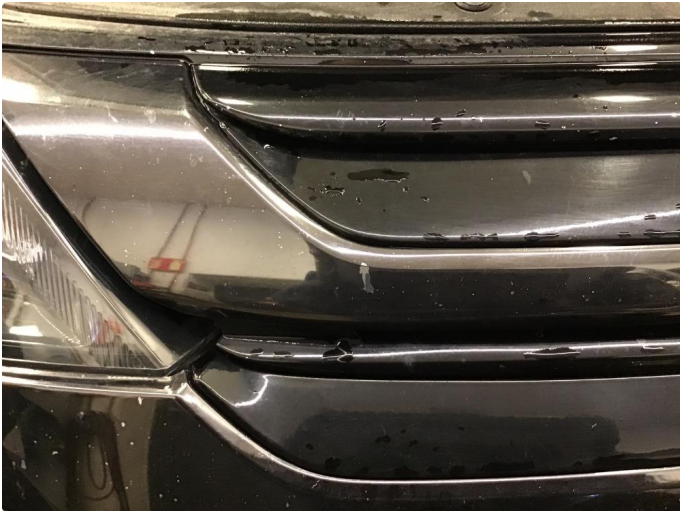
1.1 Noe lakklass grill pga steinprut.
