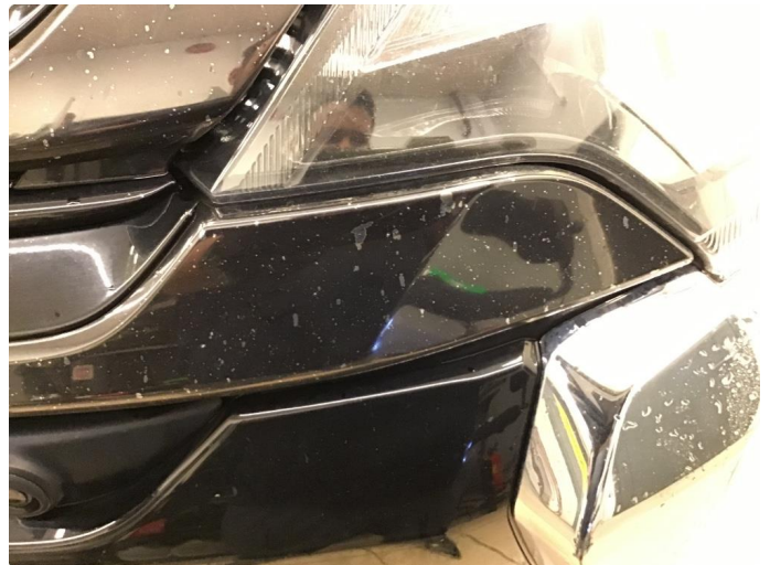
1.1 Noe lakklass grill pga steinprut.
