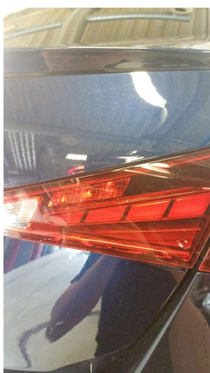
2.1 Krakelering i plast
