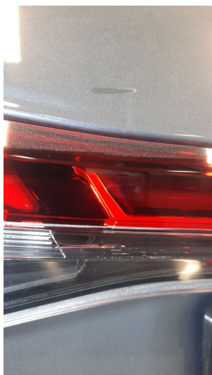
2.1 Krakelering i plast
