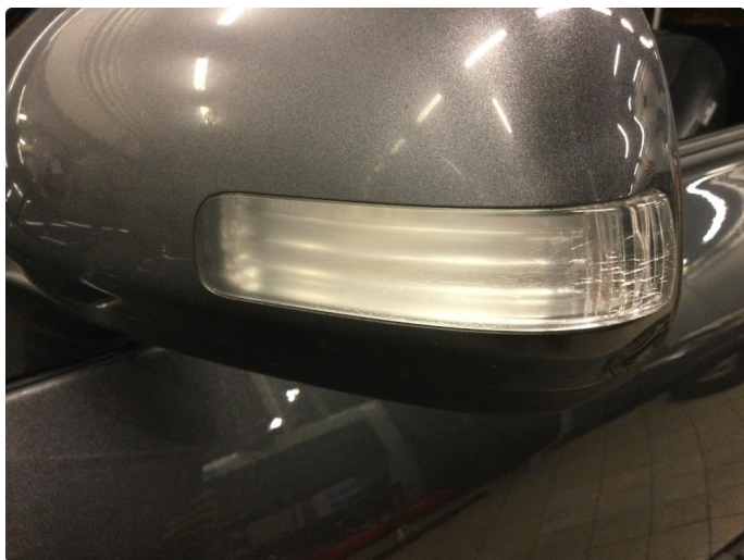
2.2 Krakelering i plast
