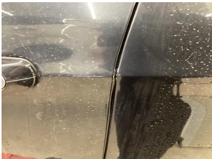
2.5 Rust i fals
