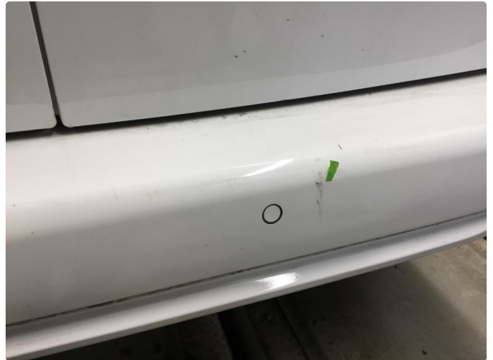
1.1 Noe riper/hakk i lakk bakfanger. Penselflekket.
