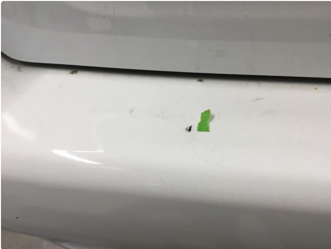
1.1 Noe riper/hakk i lakk bakfanger. Penselflekket.
