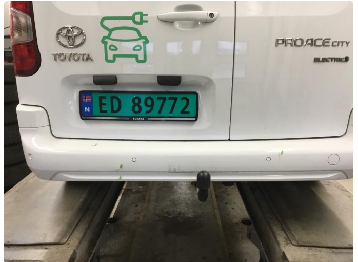
1.1 Noe riper/hakk i lakk bakfanger. Penselflekket.
