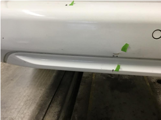
1.1 Noe riper/hakk i lakk bakfanger. Penselflekket.
