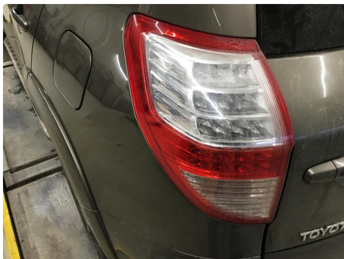
2.2 Noe dugg/fukt i v. baklampe.
