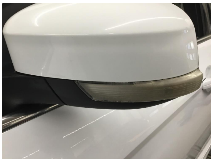
2.1 Matte glass blinklys i speil begge sider, samt noe sprekker v.side.
