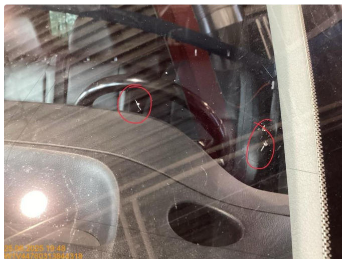
1.2 Reparert steinsprut utenfor synsfelt
