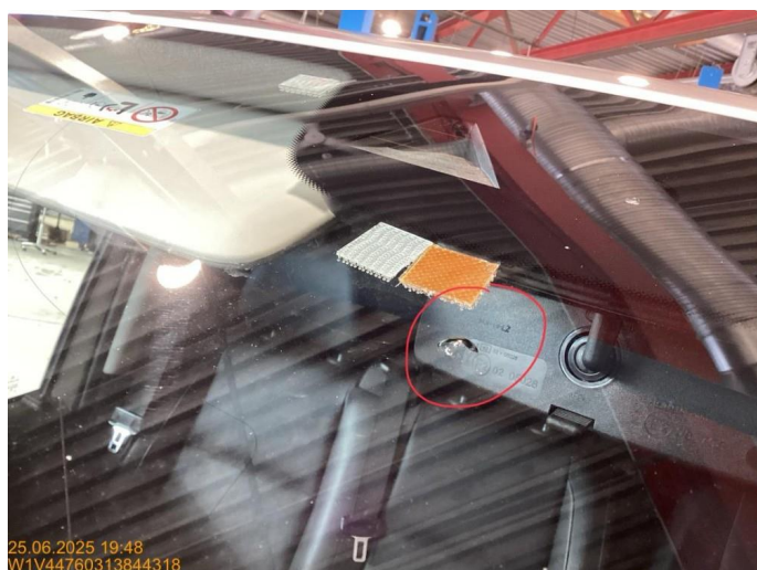
1.2 Reparert steinsprut utenfor synsfelt
