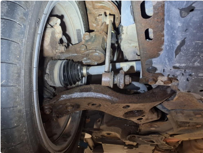
1.1 Overflaterust i understell
