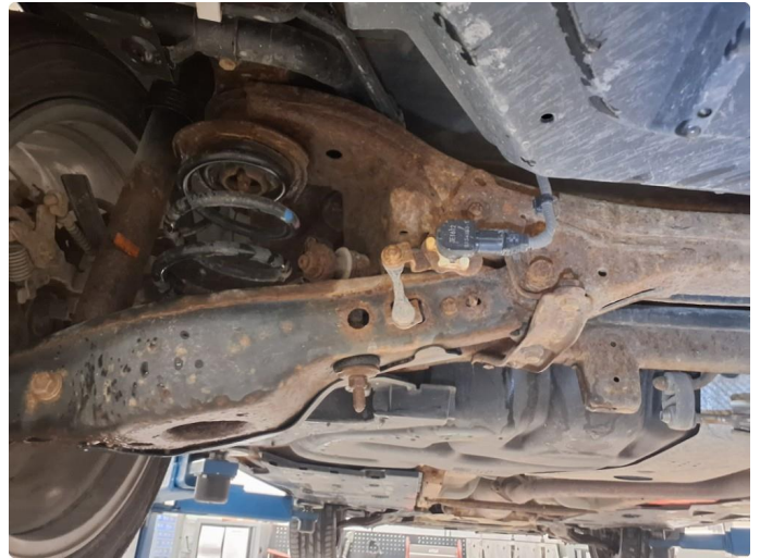
1.1 Overflaterust i understell
