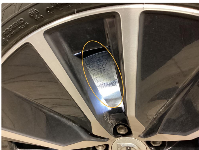
3.1 Mer enn 25% rust. OK
