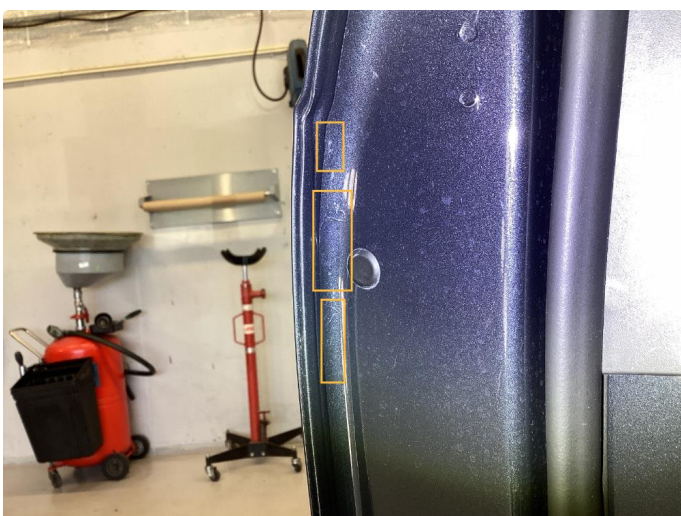
1.3 Rust i fals. Intakt
