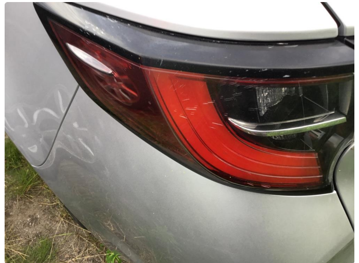
2.1 Krakelering i plast
