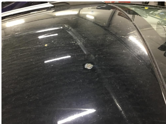
1.1 Reparert steinsprang tak
