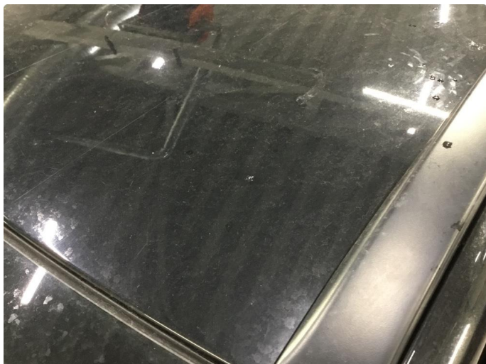
1.1 Reparert steinsprang tak
