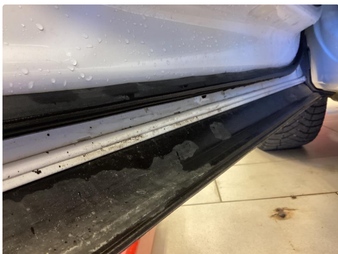
1.2 Rust i fals
