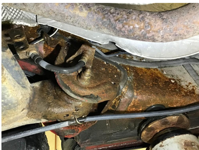
1.1 Rust underside bil.
