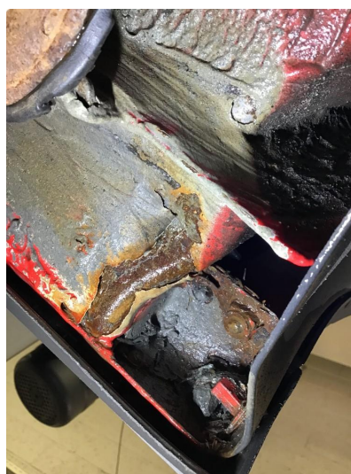
1.1 Rust underside bil.
