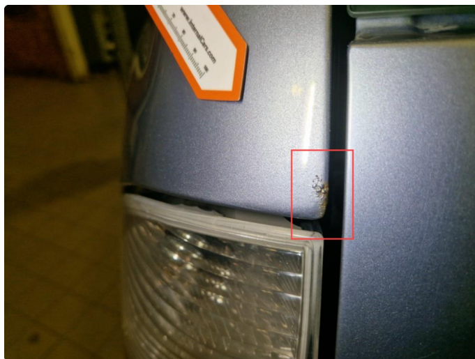
2.5 Noe rustdannelser + liten bulk v/bakskjerm.
