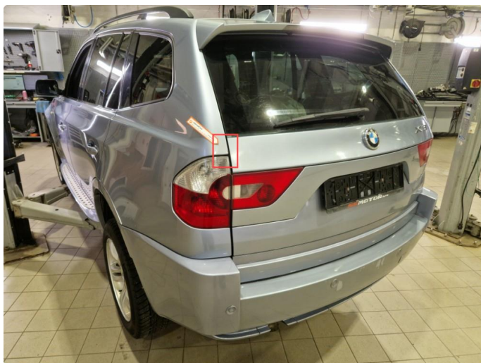
2.5 Noe rustdannelser + liten bulk v ir bakskjerm.
