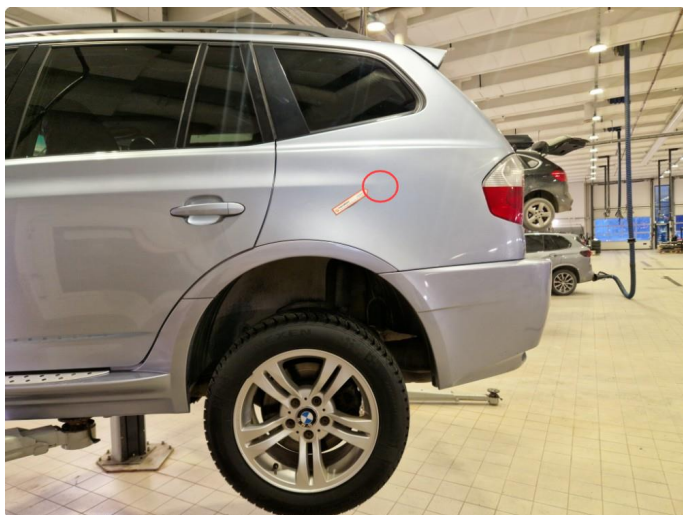
2.5 Noe rustdannelser + liten bulk v/bakskjerm.
