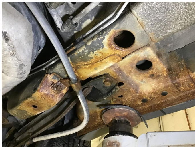
1.3 Mye rust underside bil.
