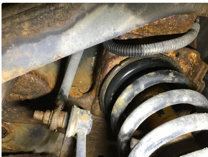
1.3 Mye rust underside bil.
