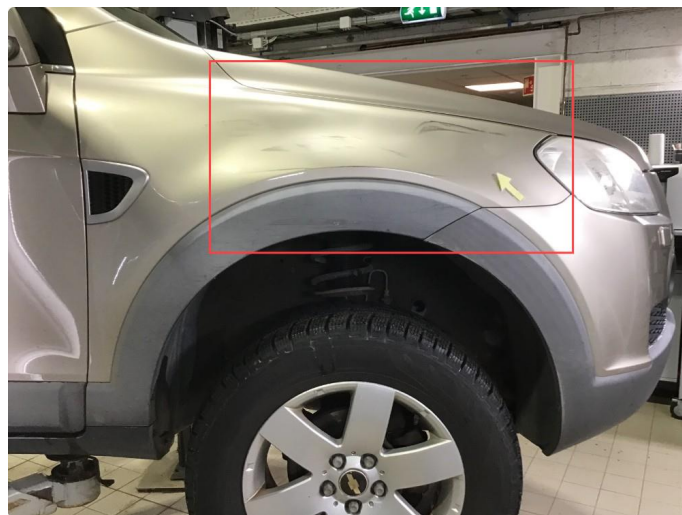
1.7 Riper / bulker h-framskjerm.
