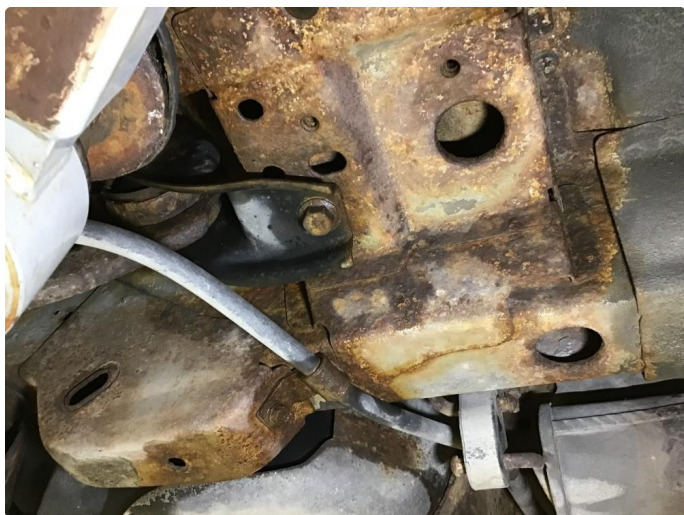
1.3 Mye rust underside bil.
