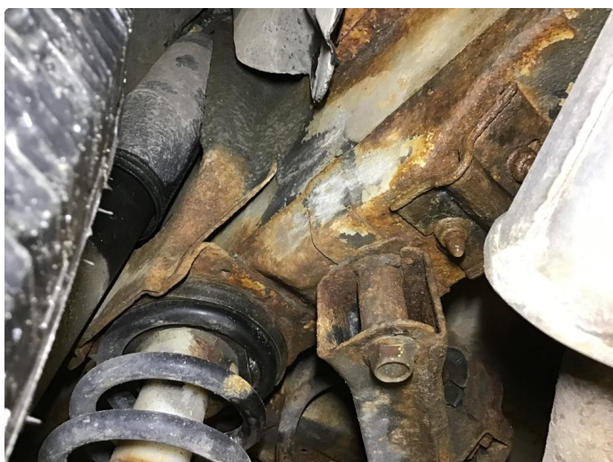
1.3 Mye rust underside bil.
