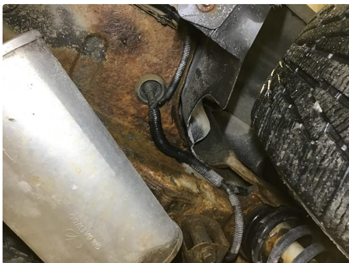
1.3 Mye rust underside bil.
