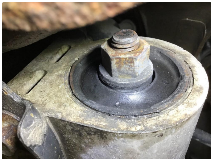
4.1 Utslitt casterforing h+v fram.
