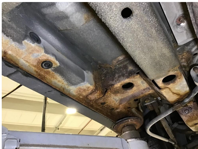
1.3 Mye rust underside bil.
