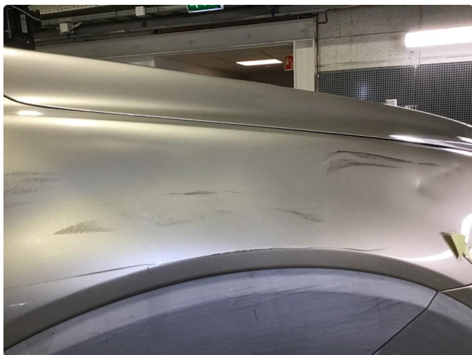
1.7 Riper / bulker h-framskjerm.
