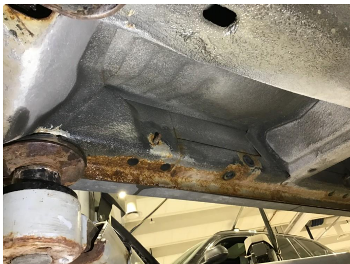
1.3 Mye rust underside bil.
