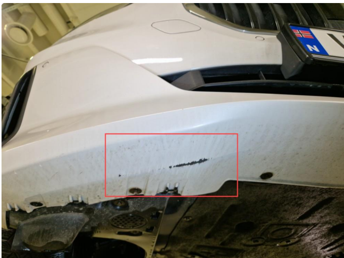
1.3 Noe skrubbermerker underkant fremfanger.
