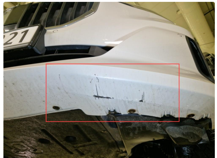
1.3 Noe skrubbermerker underkant fremfanger.
