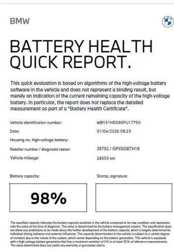
3.1 Test HV-Battery Condition OK, 98%
