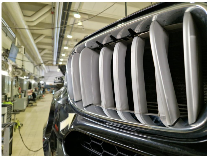
2.14 Skadet grillnyre h-side.
