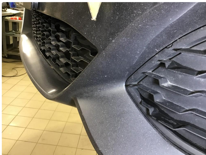
2.9 Mye lakkslitasje / riper frontfanger.
