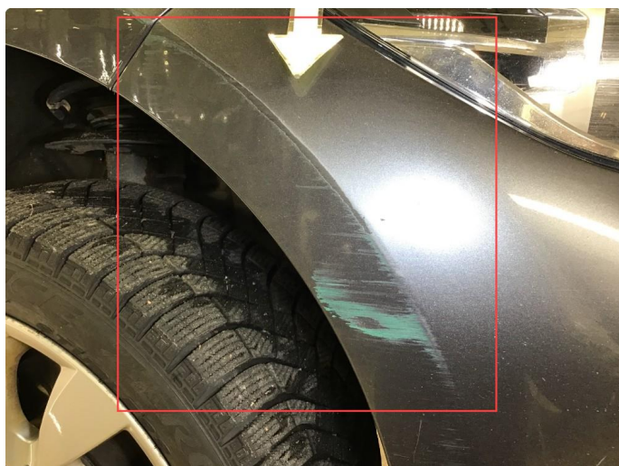
2.9 Mye lakkslitasje / riper frontfanger.
