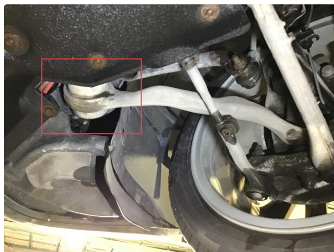
5.3 Slitte casterforinger h+v side fram.
