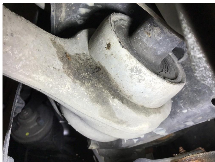
5.3 Slitte casterforinger h+v side fram.
