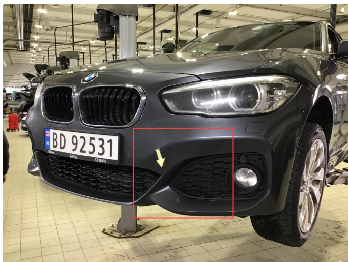
2.9 Mye lakkslitasje / riper frontfanger.
