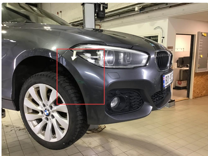
2.9 Mye lakkslitasje / riper frontfanger.
