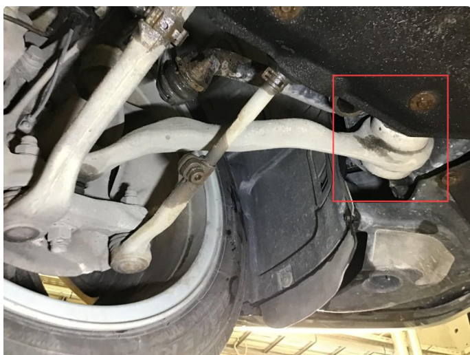
5.3 Slitte casterforinger h+v side fram.
